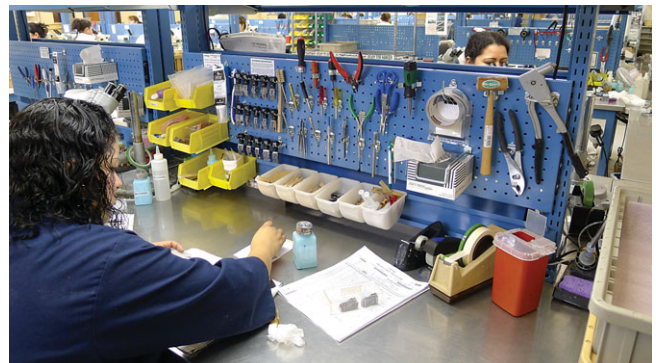
On the revamped shop floor, each station uses pegboards to organize the tools and components for operators to accomplish their tasks. Note the stainless steel work surfaces here in the epoxy potting cell. The upper shelf aggregates finished assemblies. Photo courtesy IAC Industries Inc.
