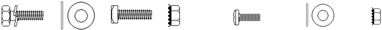
1/4-20x .75 HH Bolt 1/4-20 Flat washer 1/4-20x .75 SQ.H Bolt 1/4-20 Hex Keps Nut 10-32x 0.75L PPH Screw # 10 Flat washer #10-32 Hex Keps Nut
